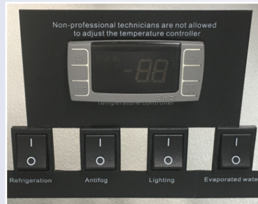
Digital controller: Temperature/ Refrigeration/ Anti-fog/ Lighting/ Evaporated water
